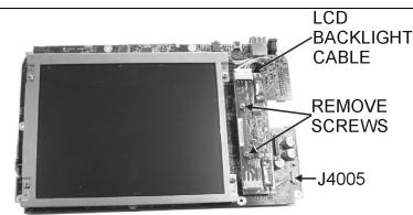
Figure 20. LCD Backlight PCB Removal and Replacement
