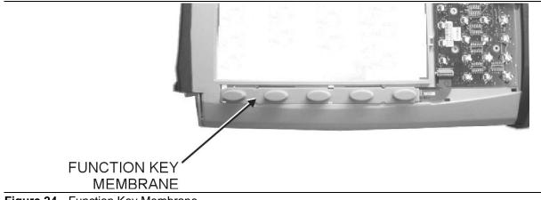
Figure 24. Function Key Membrane
