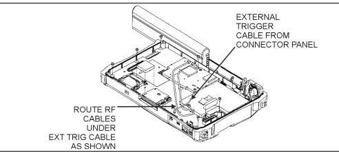
Figure 14. Cable Routing Diagram
