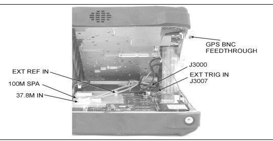
Figure 13. Front Panel Assembly Removal and Cable Connections
