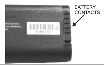
Figure 11. Battery Contacts
