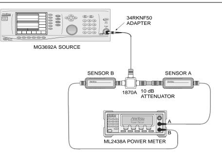
Figure 2. Level Accuracy Across Frequency Test Pre-test Setup
