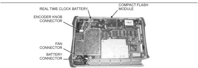
Figure 17. Main PCB Assembly Replacement
