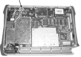
Figure 15. RTC Lithium Battery on the Main PCB
