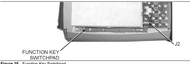
Figure 25. Function Key Switchpad
