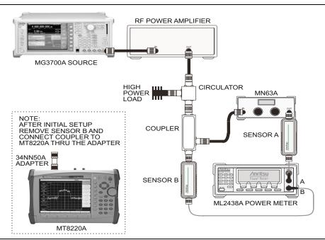
Figure 5. W-CDMA Absolute Power Accuracy Test Setup
