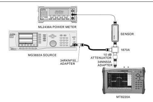
Figure 3. Level Accuracy Across Frequency Test Setup
