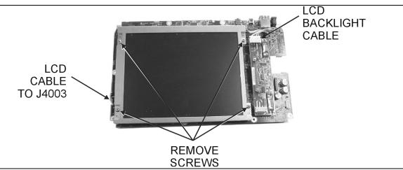
Figure 19. LCD Assembly Replacement
